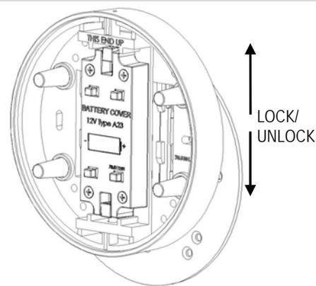
To attach the housing to the mounting plate, place the housing over the mounting keys on the mounting plate, and then slide the housing downward until the locking tab engages the housing. To remove the housing, press in the locking tab and reverse this procedure. To securely lock the plate, put an additional screw through both the housing and the mounting plate.
