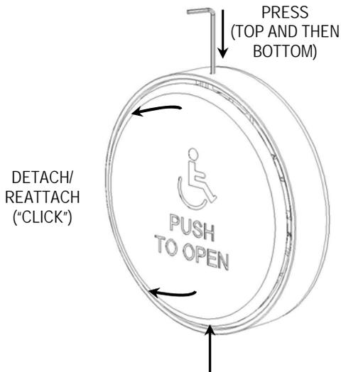
To assemble or disassemble the push plate, use the enclosed hex key (or similar diameter tool) to press in and release the spring clips from the faceplate bracket. The spring clip will need to be engaged / disengaged from top and bottom, one at a time. When the spring clips are correctly engaged, they will make a "click". It may be necessary to rotate the faceplate slightly to have them lock correctly.
